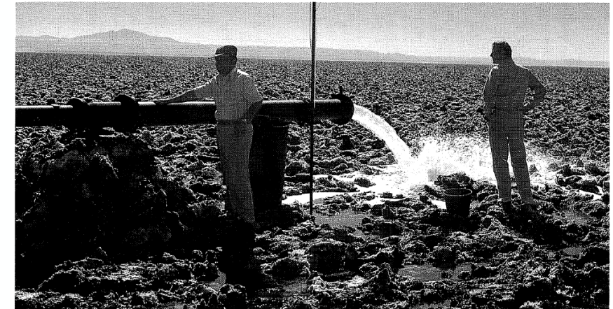
Among other things, Foote needed to know how much brine lay underground. In a test that would help answer that question, brine, here shown gushing from the pipe, was pumped out of one well at the rate of a thousand gallons per minute without letup for three months. Even after all that drain, the level in the well had declined only slightly.
